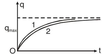
**D 11\*** The instantaneous charge on a capacitor in two discharging RC circuits is plotted with respect to time in figure. Choose the correct statement(s) (where  $E_1$  and  $E_2$  are emf of two DC sources in two different charging circuits).
