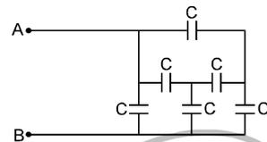
**C 30.** In the battery of capacitors shown, all the capacitors have equal capacitances. Then the equivalent capacitance of the system across the terminals A and B :
