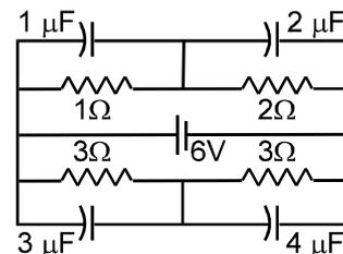
**B 5.** (i) Find the charge supplied by the battery in the arrangement shown in figure.
