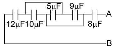
**C 29.** The equivalent capacitance between point A and B is
